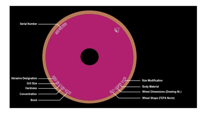
The number following the wheel shape (FEPA), determines all the dimensions of the wheel, also we add additional space regards size modification (e.g.: an angle).
