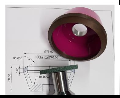
The 11V5R type is especially developed for the Walter Micro machine.
